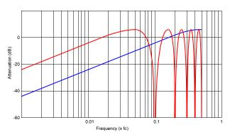
Shown above is the weighting function (difference compared to a reference-based measurement) implicitly applied by the period jitter (n=1) and long-term jitter (n=10) procedures.
