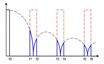
Sensitive areas are DC to  $2 \cdot f_{max}$  and all its aliases. Total noise level relative to the test signal at fmax is found by integrating noise power across each band and summing all of these.
