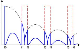
More often than not, the noise shaper runs substantially faster than he upsampling filter. In this case, the sinc function is applied to the noise spectrum separately and scaled corresponding to its sample rate (shown below is a situation where the noise shaper runs four times faster than the filter).
