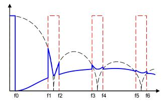
The noise contribution by the jitter breaks down into two parts. One is associated with demodulating aliases and is analysed as 5.1. The other part comes with the shaped noise. If the SNR requirement of a converter is more stringent than THD+N, the latter is considered alone.
